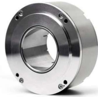
A110H is a photoelectric hollow shaft angle encoder that produces up to 1.800.000 output pulses per revolution and has the accuracy of ±5 arc. sec.
