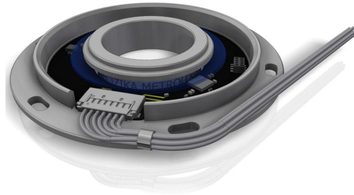
This is a high-resolution, singleturn absolute encoder kit with a 22 Bit BiSS-C interface. The encoder consists of several optical reflectance sensors arranged at an angle of 180 degrees to each other.
