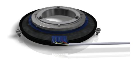
This is a high-resolution, singleturn absolute encoder with a 22 Bit BiSS-C interface. The encoder consists of several optical reflectance sensors arranged at an angle of 180 degrees to each other. This allows to
