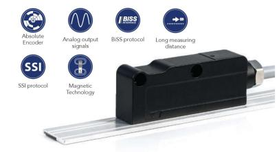
Magnetic absolute linear encoder MK has measuring length of up to 30.000 mm, accuracy can reach up to  $\pm35~\mu m$ . The encoder has two versions of serial interface - SSI or BiSS C, but optionally it can
